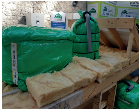
Example of Insulated tanks and pipework
